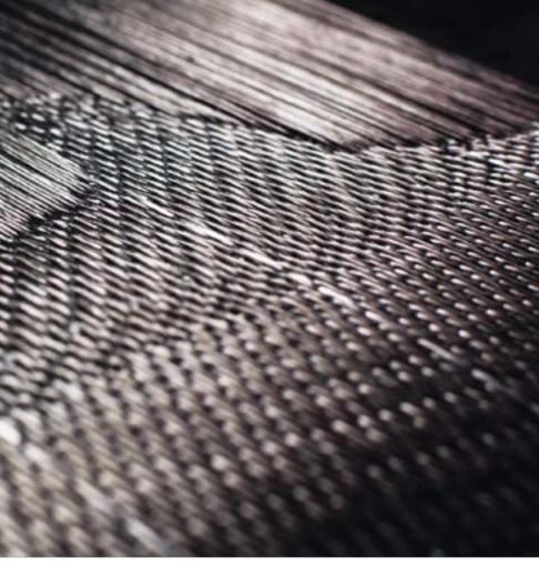
• The 3-D woven RTM (Resin Transfer Molding) carbon fiber composites used for the fan blades and fan case on the LEAP engine are revolutionizing the single-aisle market.
