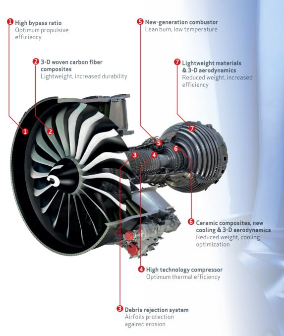
CFM 'S LEAP ENGINE IS AN IMPRESSIVE PACKAGE OF INNOVATIVE TECHNOLOGIES. IT SETS A NEW STANDARD IN ENGINES FOR SINGLE-AISLE COMMERCIAL JETS, PROVIDING A 15% REDUCTION IN FUEL CONSUMPTION AND CO<sub>2</sub> EMISSIONS VERSUS PREVIOUS GENERATION ENGINES.
